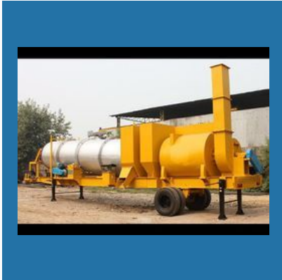
Mobile Asphalt Drum Mix Plant
