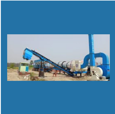
Asphalt Hot Mix Plant
